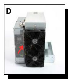
Slide the old power supply off the chassis, as shown in Figure E.
